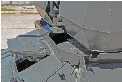
That big black rectangular cutout in the chassis is flame-cut and unfinished! That was the ammo reload point.
