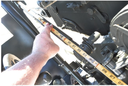
A simple expanding ruler gives me the numbers I need to replicate this part... whatever it might be. A vernier caliper will give me diameters.
