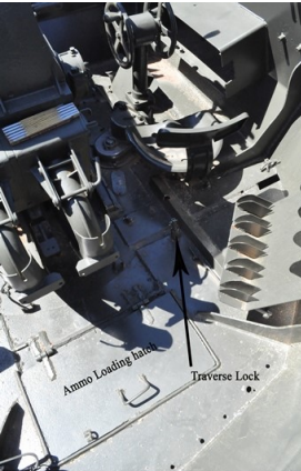
To replenish ammo from the interior of the tank, the crew would rotate the cupola to line the ammo loading hatch with the cutout in the tank chassis. The traverse lock prevented the cupola from rotating during ammo reloads. The traverse lock aligns (one assumes) with a hole drilled into the front left of the chassis.
